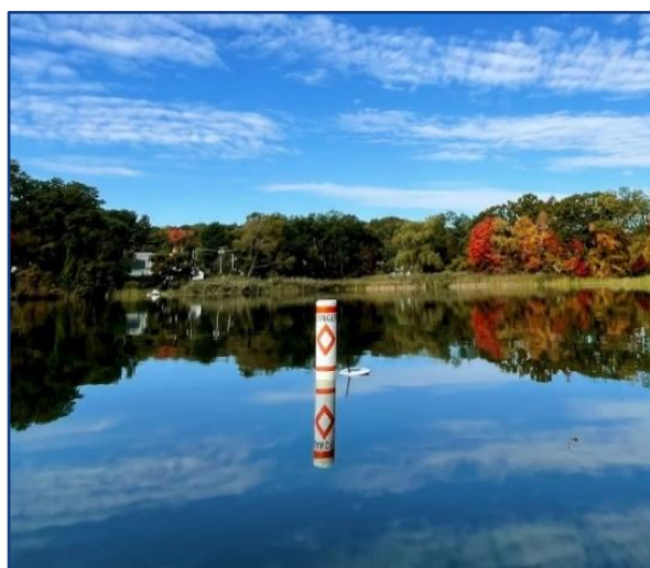
Figure 13 – A continuous monitoring buoy was deployed to track cyanobacteria indicators in the northern cove of Indian Lake.
