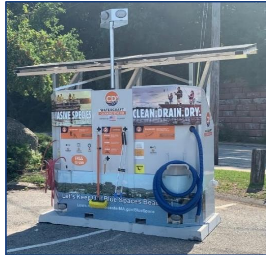
Figure 16 - Solar powered boat decontamination stations were installed at Indian Lake and Coes Reservoir to enable lake goers to decontaminate their watercraft before and after use to avoid transporting invasive plants between lakes.
