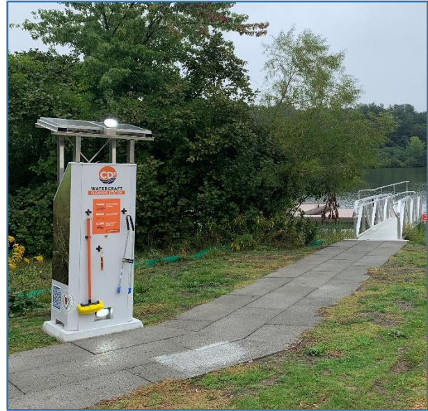
Figure 23 - Solar powered boat decontamination stations were installed at Coes Reservoir to help enable boaters to stop invasive plants at the source by decontaminating watercraft before and after use.
