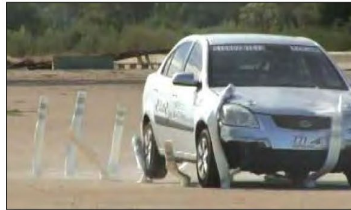
City Posts rebound back to their original position, even after more than 100 high-speed hits on the TTI Test Deck
