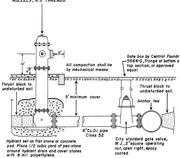
No. Rev. Ву Date HYDRANT DETAIL MJF 5/5/78 H/28/80 Typical 2/7/91 3/31/97 AVC CITY of WORCESTER AVC 12/28/00 DETAIL Drawn by: R.H. & AV.C. DEPARTMENT of PUBLIC WORKS NO SCALE Checked by: A.C.M. **W-9** WATER OPERATIONS Date: 2/24/78
