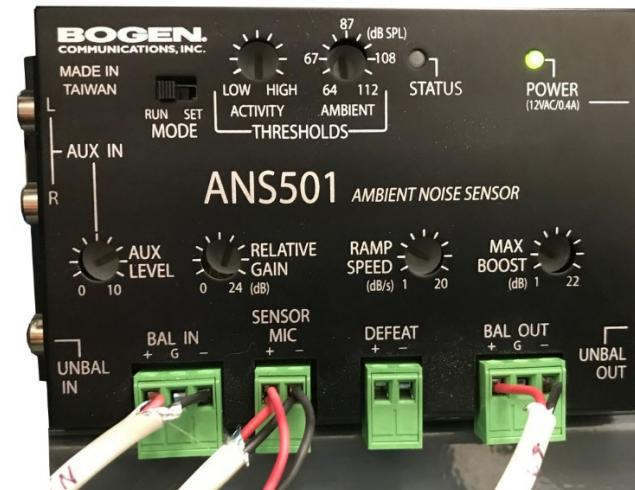
Fig 3 – ANS501 Control Unit Wiring
