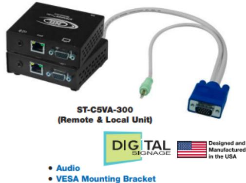
The XTENDEX® VGA Extender transmits VGA video up to 300 feet away from a computer using CAT5/5e/6/6a cable. Each video extender consists of a local unit that connects to a computer and also supplies video to a local monitor, and a remote unit that connects to a monitor.
