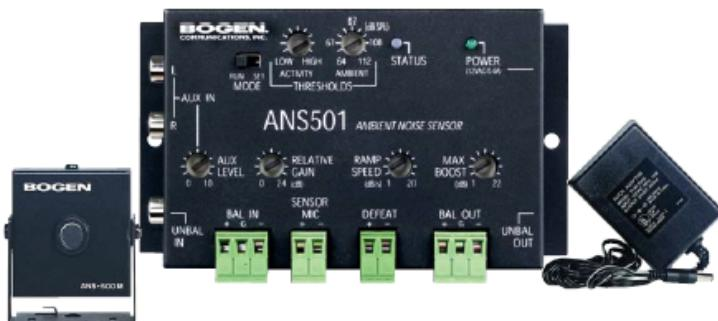
**Description** The Bogen Ambient Noise Sensor system is designed to monitor continuously changing ambient noise levels and electronically adjust the level of a page announcement and/or background music so intelligibility is maintained. The system consists of the control module (Model ANS501), a microphone module (ANS500M), and a power supply.
