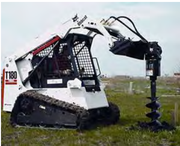
Skid Loader with Auger attachments
