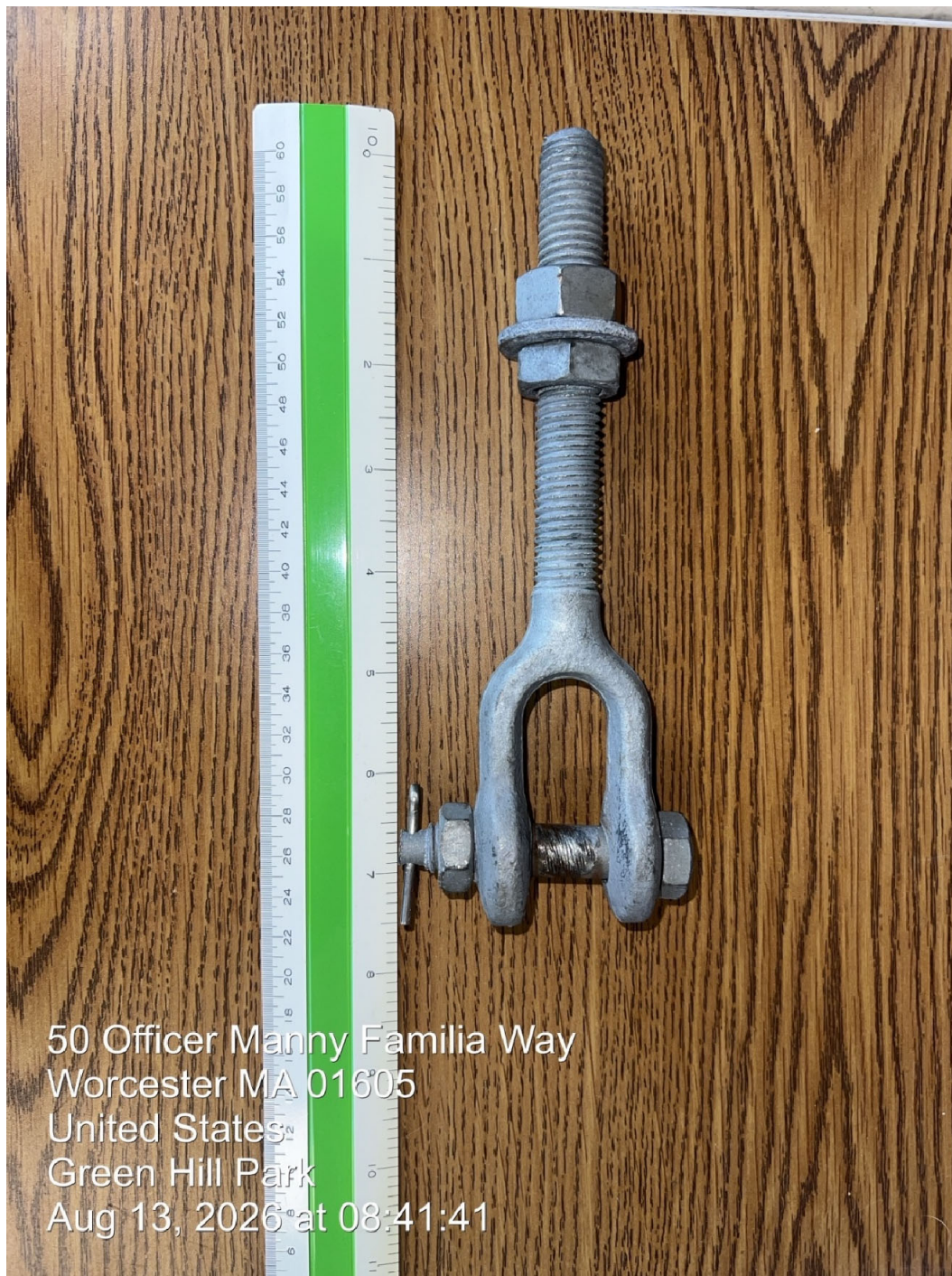
Figure 3: Existing jaw assembly, approximately 7.5 inches in length. Include in quote to furnish (from Manufacturer of Shade Structure) and install new and complete jaw assembly for Model QRE fabric.
