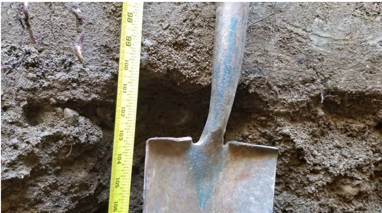
Photo 2 - TP-1 - Depth to bottom of foundation
