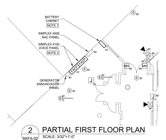
WORCESTER UNION STATION 02/29/24 DATE: FIRE ALARM CONTROL PANEL REPLACEMENT SCALE: AS NOTED FIRST FLOOR PLANS DRAWN: MWF Hallam<sup>®</sup>ICS MWF CHECK: PROJ. NO. 23343.000
