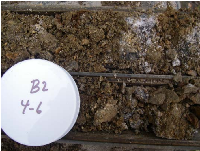
Photo 3: Granular Fill (AR) in B2 at 4 ft.
