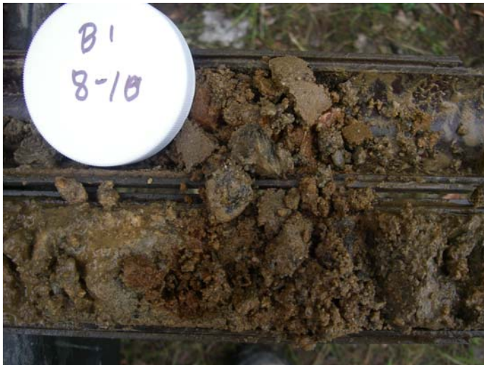
Photo 5: Water in Ablation Till (GT) in B1 at 8 ft.
