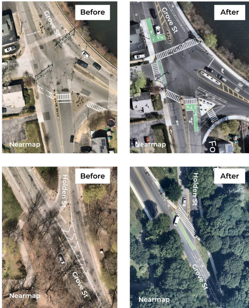
Figure 12: Before and after photos of Grove Street showing changes to intersections and the addition of bike lanes
