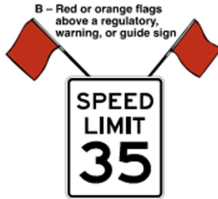
Figure 2A-1. Examples of Enhanced Conspicuity for Signs
