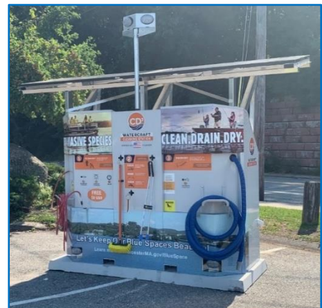
Figure 13 - Solar powered boat decontamination stations were installed at Indian Lake and Coes Reservoir to enable lake goers to decontaminate their watercraft before and after use to avoid transporting invasive plants to the lakes.
