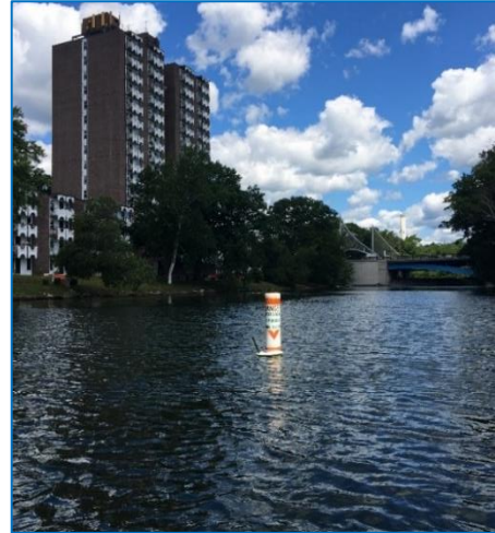
Figure 21 – A continuous monitoring buoy was relocated just south of the Route 9 Outfall to track possible effects from increased disturbances over the past year.
