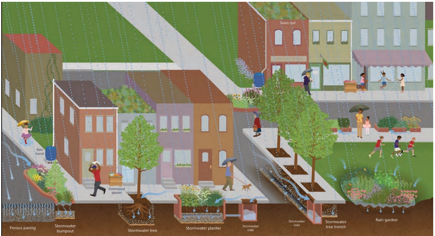
Urban Green Infrastructure Installations (Philadelphia Clean Waters, Green City)
