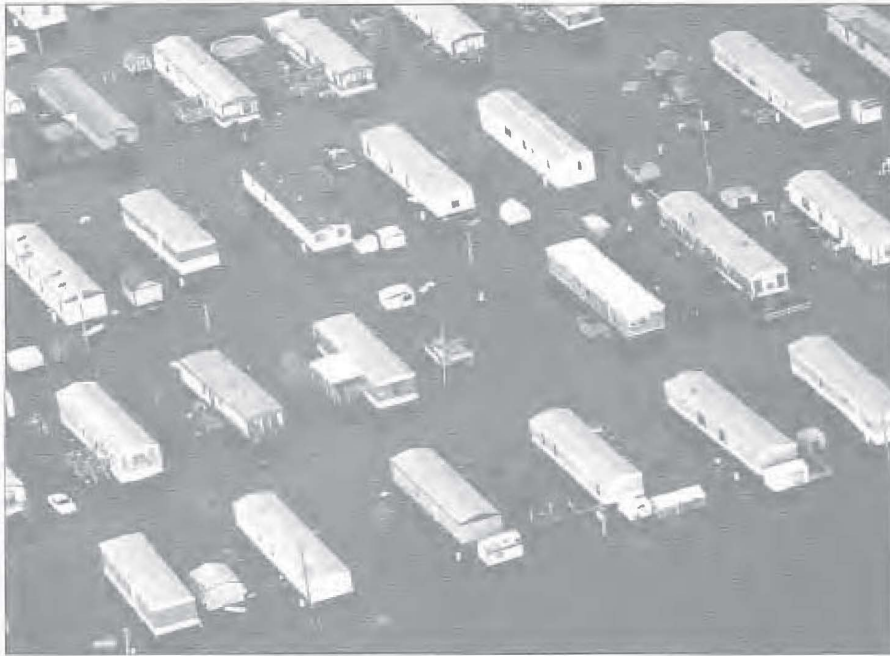
Figure 3a - The cost-effectiveness of reducing flood losses by elevating or relocating homes was dramatically demonstrated in parts of the Midwest in June, 1995. The top photograph shows an inundated mobile home park along the Missouri River during the Great Flood of '93. The same area flooded again in 1995 (bottom photograph, as the floodwaters were rising), but there was little flood damage because the families had been moved to new safe sites. Some 10,000 homes in the Midwest have been elevated, relocated, or acquired with Federal and state funds since 1993.
