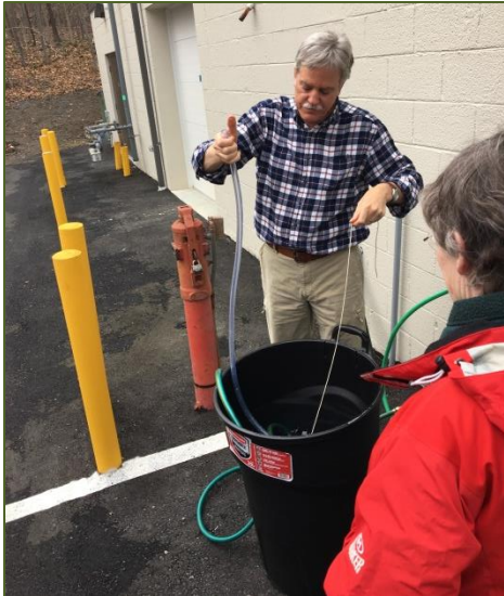
Integrated tubes allow us to sample 3 m of water. Here we practice collecting them in a barrel.
